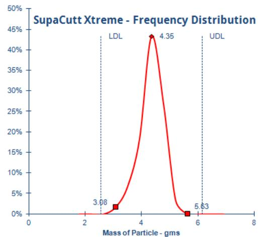
SupaCutt Xtreme fragments are very consistent in size as shown on the distribution graph. Above 80% of the fragments being within a 10% spread of mass. The uniformity of the fragments ensures an even cutting structure with no wastage of small or over sized fragments.
